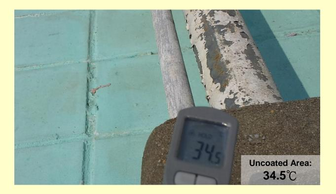
Temp. Test: After Roof Heat Rejected Coating was applied
